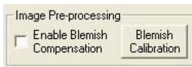
FIGURE 22. Checking “Enable Blemish Compensation” activates Image Pre-Processing.
